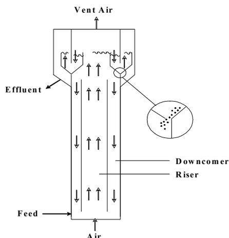
Figure 3. The Aerobic Bio-reactor
